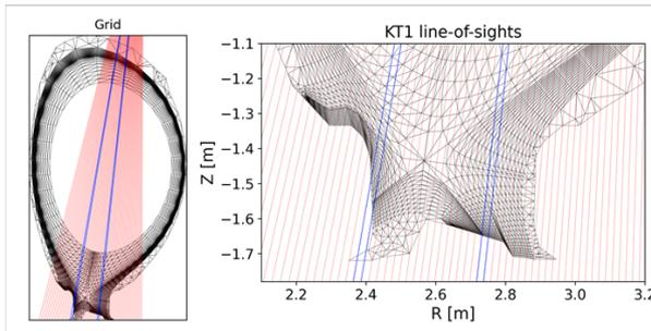
← Sight lines of the vertically viewing scanning mirror VUV-vis imaging spectroscopy system (KT1) in JET-ILW superimposed on the SOLPS-ITER grid. Blue lines are strike point locations.
