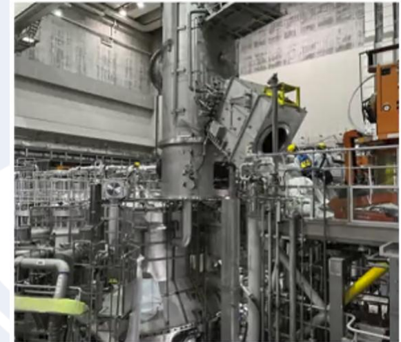
Tanks of perpendicular NBI reinstalled in the torus hall
