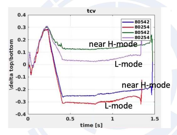
H-mode access at different values of upper δ established in TCV for AUG new shape development for 2025
