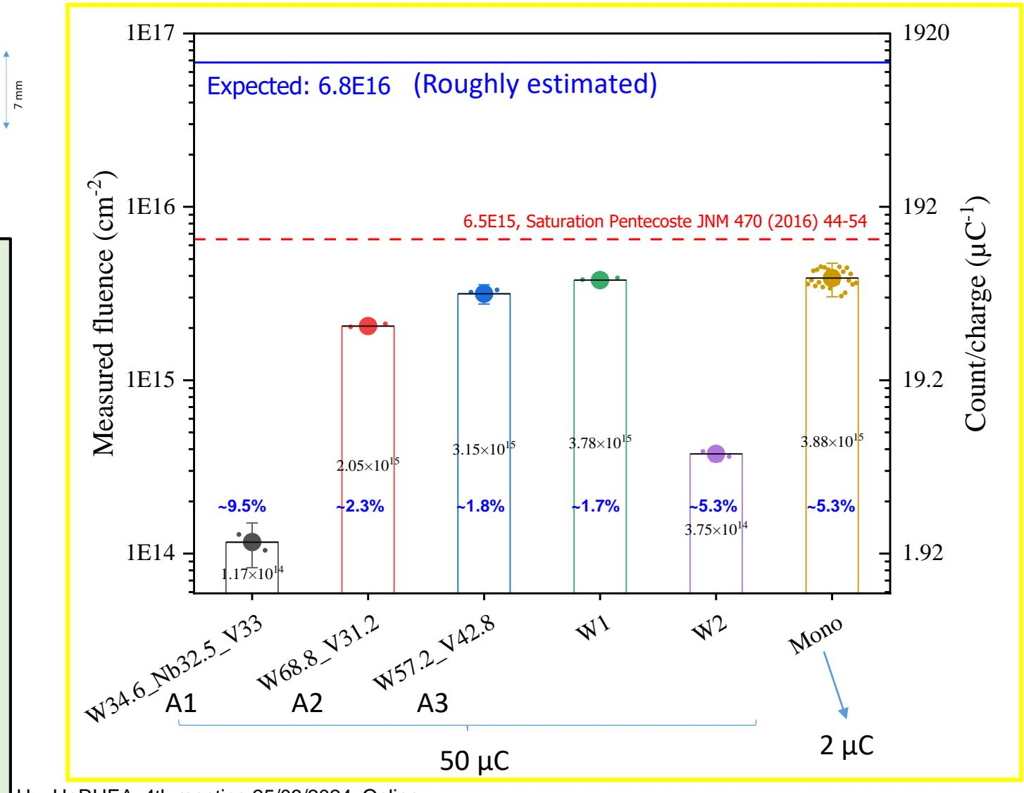
HEAs thin layers/ MgO substrate: A1(W34.6-Nb32.5-V33), A2(W68.8-V31.2), A3(W57.2-V42.8), pure W<sub>1</sub>, W<sub>2</sub>
