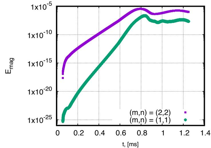
**Figure 4:** Time evolution of magnetic energy for two modes, showing distinct growth rates and nonlinear saturation behaviour.
