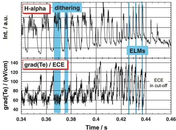
**Figure 6:** Behaviour of plasma edge parameters during a transition to H mode [Hirsch, M., et al. *Plasma Physics and Controlled Fusion* 42.5A (2000): A231].
