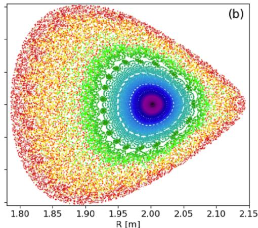
**Figure 2:** Though the degree of ergodization varies over the simulation time, the plasma core survives even the period of worst confinement (b,  $t = 0.421$  ms) [R. Ramasamy, K. Aleynikova, Nikita Nikulsin, et al. *Nuclear Fusion* 64, no. 8, 086030 (2024)].
