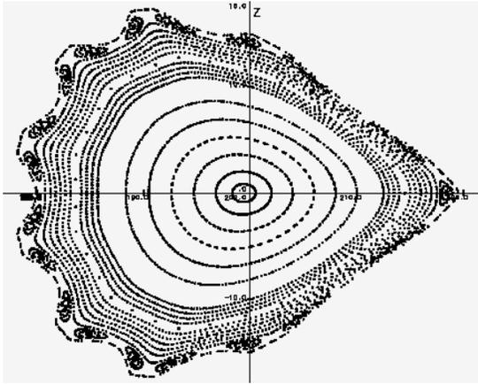
**Figure 5:** Poincaré plot (vacuum case) of the magnetic surfaces in W7-AS; island structures can form at the plasma edge, making it harder for the edge transport barrier to develop. [Hirsch, M., et al. *Plasma Physics and Controlled Fusion* 42.5A (2000): A231].
