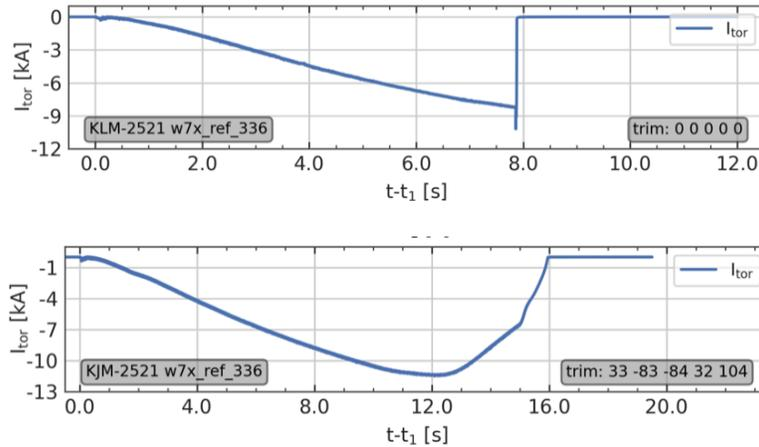
**Figure 3:** Toroidal current vs time, termination dynamics in W7-X, different configurations and different ECCD settings.
