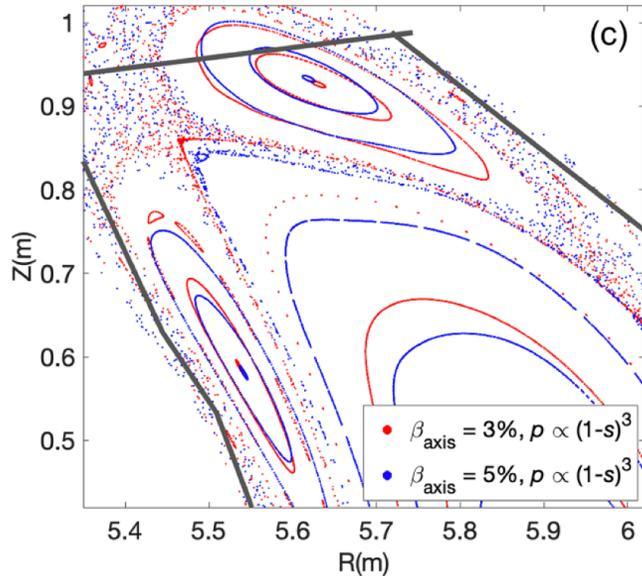
**Figure 7:** Poincaré plot illustrating a poloidal shift of the magnetic island due to finite-beta effects [S. Xu, Y. Liang, A. Knieps, S. Zhou, Y. Feng, D. Reiter, Y. Suzuki, M. Jia, J. Geiger, F. Reimold et al., *Nuclear Fusion*, vol. 63, no. 6, 066005 (2023)].
