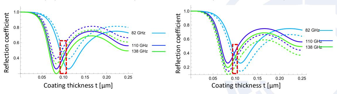
The two curves for each frequency correspond to perpendicular (solid line) and 45° (dashed line) incidence
