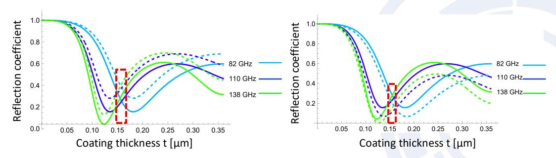
The two curves for each frequency correspond to perpendicular (solid line) and 45° (dashed line) incidence
