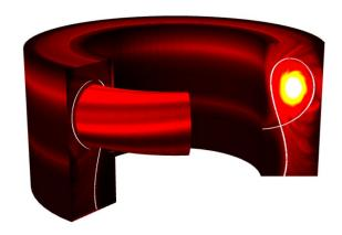
KINetic Deterministic NEutral Solver (KINDNES) - A kinetic neutrals solver that avoids Monte Carlo noise for turbulent simulations in magnetic confinement devices
