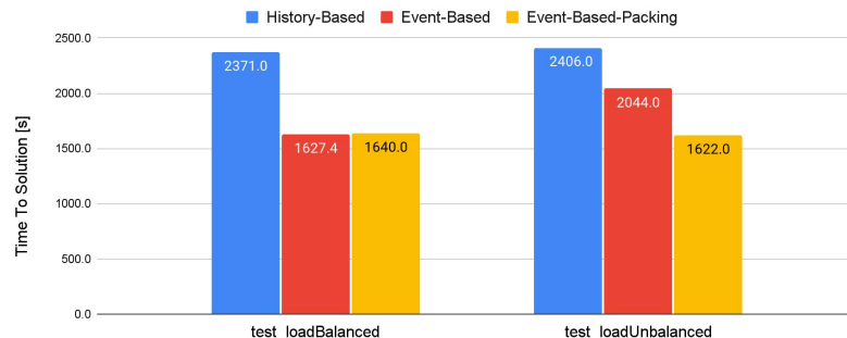
Comparison of the 3 particle-following GPU implementations - 10 Millions markers - 4 A100
