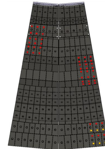
P9 → 16 triple probes on DOME + OC
