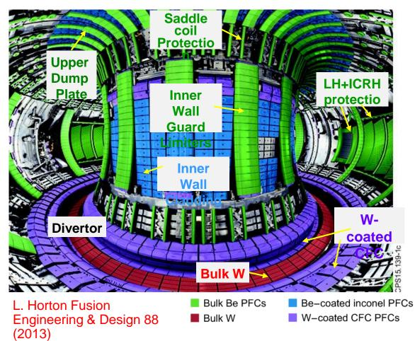
The risk of damaging the metallic PFCs caused by beryllium melting or cracking of tungsten. Significant risk of damage to the wall mitigated by multiple strategies, including a real time protection system comprising newly installed imaging diagnostics, real time algorithms for hot spot detection and alarm-handling strategy.
