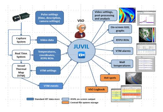
To simplify the job of the VSO, some new features, the so-called **VSO tools**, were integrated into JUVIL for the interpretation of VTM events and for the quick post-pulse analysis of video data required for the preparation of the next pulse.
