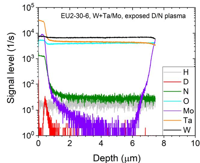
Examples of SIMS depth profiles from W-Ta sample resulting from exposure to D and D+N plasmas
