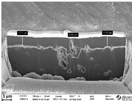
SEM image of the A191 tile with visible Mo marker interlayer and erosion of deposited C
