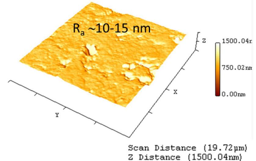
Fig. 1. As received polished SIGRAFINE® R6710 graphite -AFM analysis
