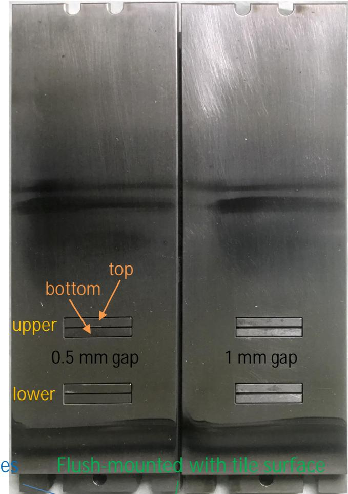
Positions of analyses before and after exposure
