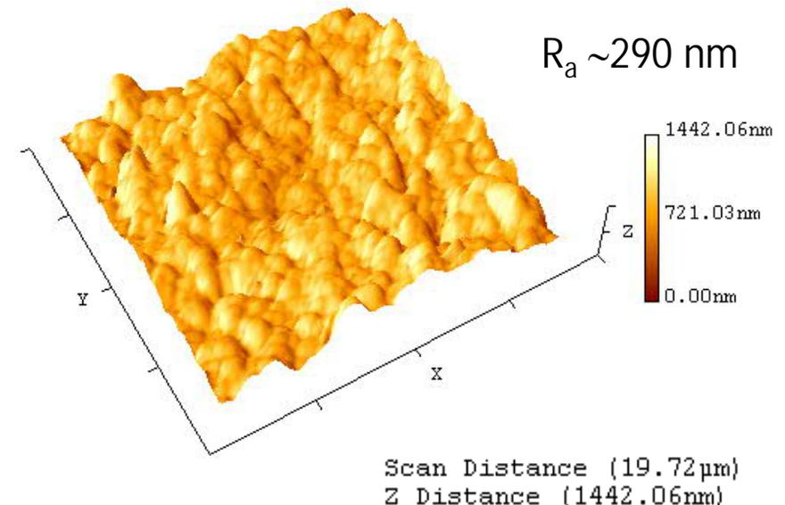
Fig. 2. Plasma treated graphite (etching for 90 min)
