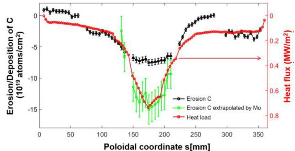
Erosion/deposition of C during OP1.2a based on ps-LIBS.
