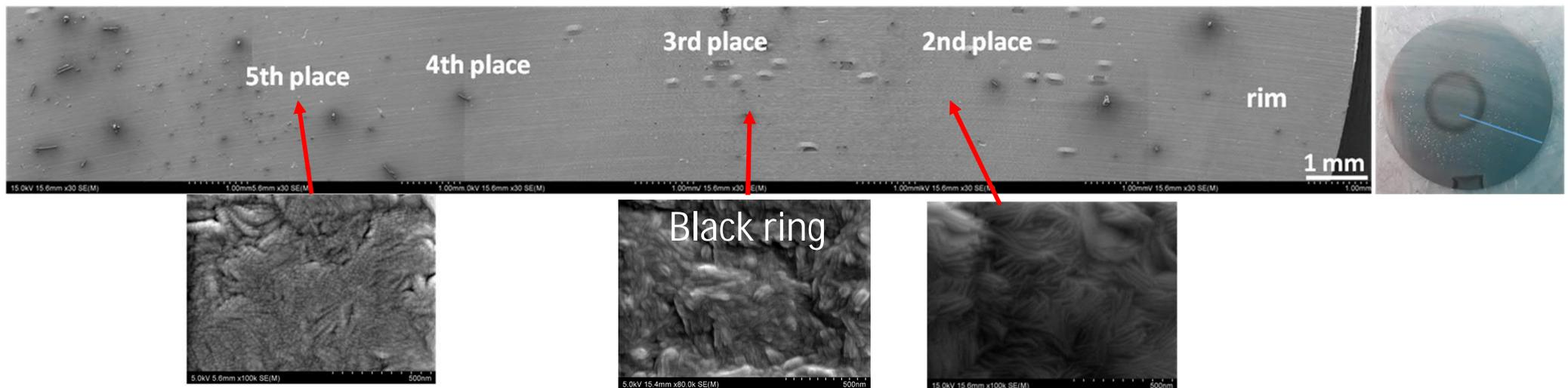
Examples of SEM images from a W-Ta sample resulting from exposure to D plasma
