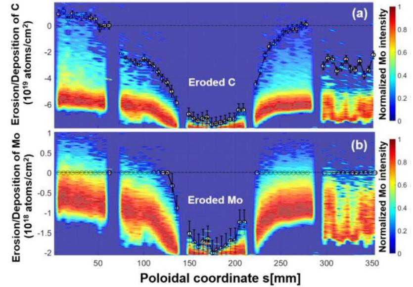
Erosion of C (a) and Mo (b) of the target element TM2v2 by ps-LIBS (OP1.2a campaign).
