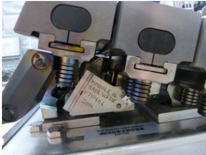
Photograph showing location of W-sticking monitor on 14W tile 5 Photograph from 2014 installation
