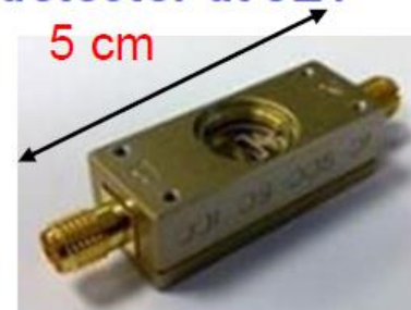
Standalone oblique diamond detector at JET
