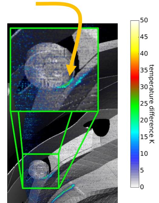
power loads in excess of 1.5MW/m<sup>2</sup> measured
