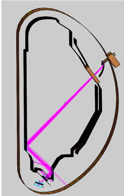
Simplified representation stabilizing plate and the sub-divertor region (cryopumps location).
