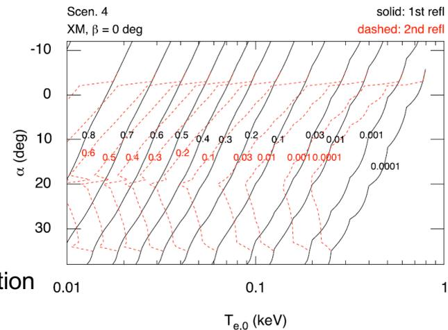
EC injection in a condition of zero (pre-ionization and ECWC experiments) or very low fraction of absorbed power  $\sim 0.1$  (assisted burn-through experiments) results in  $P \geq 0.9 P_0$  hitting the inner wall at the first pass, with **several MW/m<sup>2</sup>** per injected beam.
