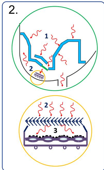
$P_{\text{stray}}=150 \text{ kW}^*$ , water baffle uncoated;  $\alpha = 0.04$
