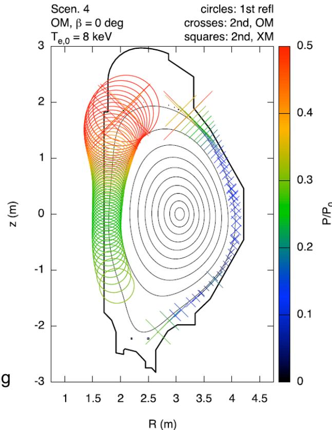
GRAY simulation of residual EC distribution and with  $T_e$  down-scaling.
